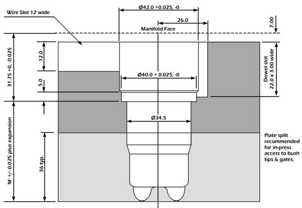
'M' = 'L' - 31.75. The expansion of the bush relative to the mould is calculated by the formula: ('L' mm minus 10) x 0.0000126 x (processing temp. °C minus mould temperature °C)
