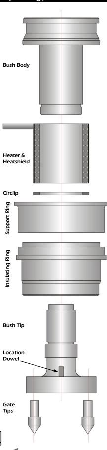
The MT32 components are identical in diameter, and differ only in length.
